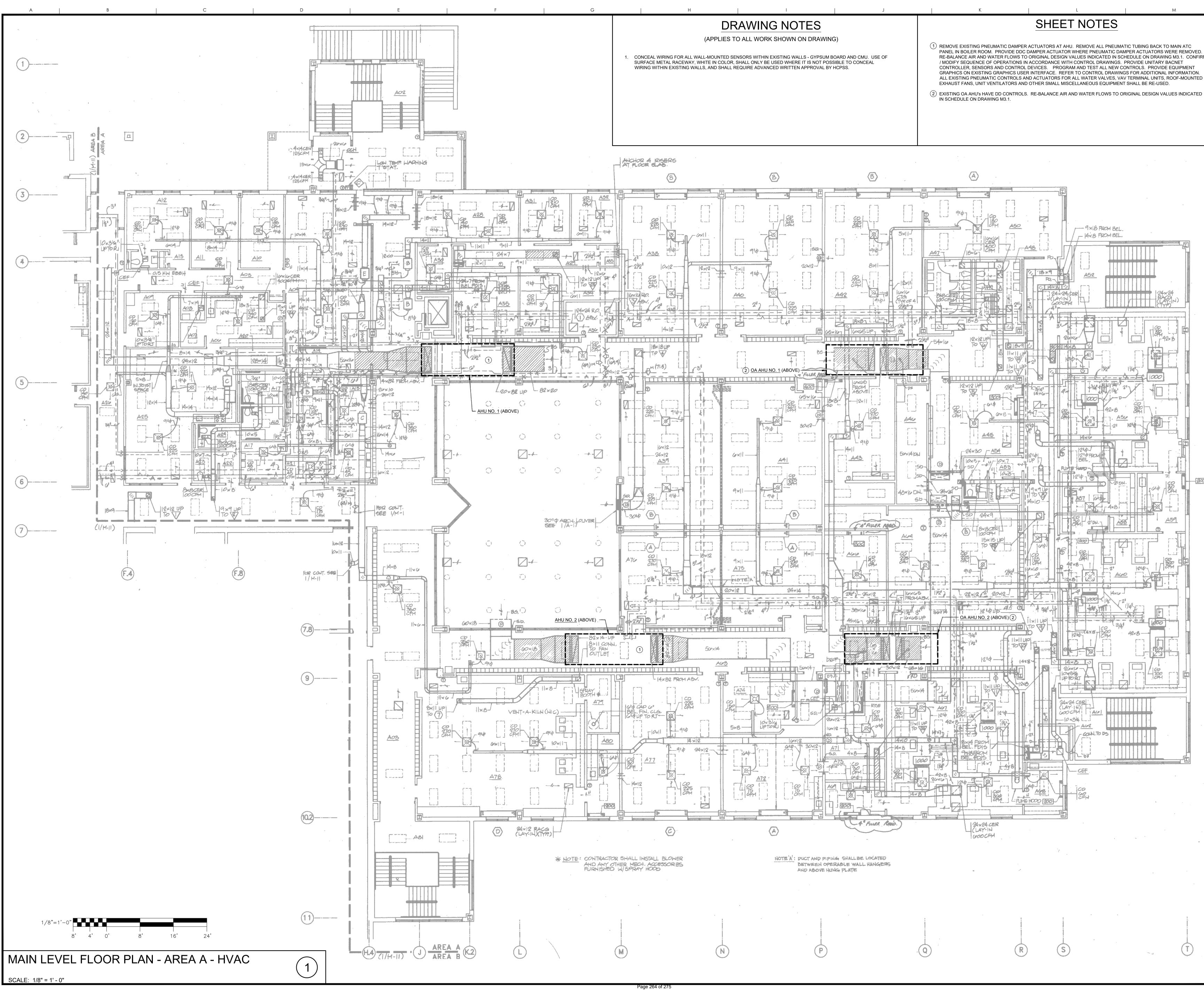
PANEL IN BOILER ROOM. PROVIDE DDC DAMPER ACTUATOR WHERE PNEUMATIC DAMPER ACTUATORS WERE REMOVED. RE-BALANCE AIR AND WATER FLOWS TO ORIGINAL DESIGN VALUES INDICATED IN SCHEDULE ON DRAWING M3.1. CONFIRM GRAPHICS ON EXISTING GRAPHICS USER INTERFACE. REFER TO CONTROL DRAWINGS FOR ADDITIONAL INFORMATION. ALL EXISTING PNEUMATIC CONTROLS AND ACTUATORS FOR ALL WATER VALVES, VAV TERMINAL UNITS, ROOF-MOUNTED
